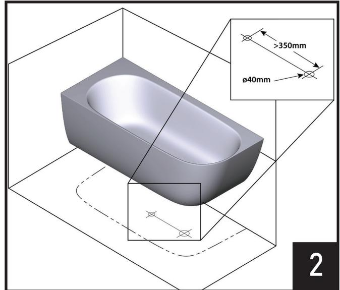
Mark accordingly on floor surface for appropriate waste drain installation connections. Note the inset diagram for waste drain measurements.
