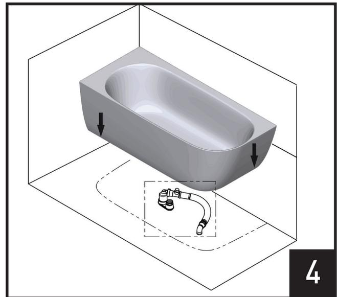
Install bathtub K36 waste drain. Install bathtub and align drain with floor waste drain.
