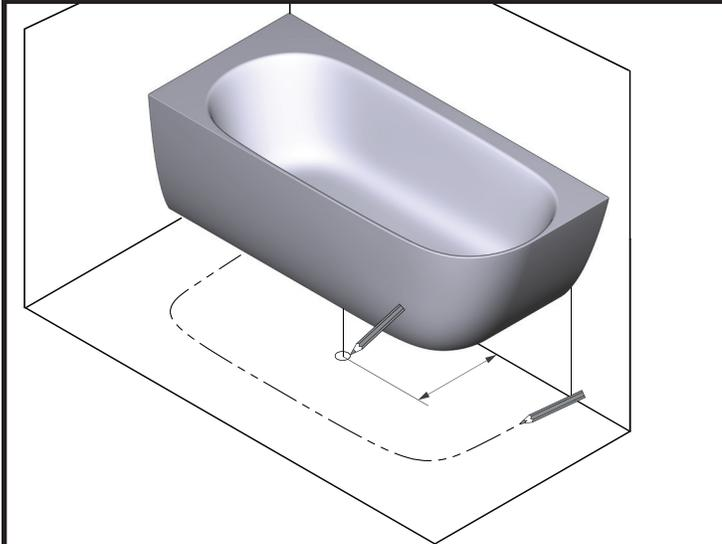
Prepare bathtub floor surface by tracing bathtub bottom edge for installation position.
