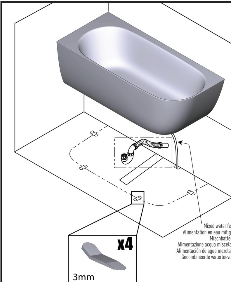
Install bathtub K60 waste drain into floor surface. Position the bathtub spacers (x4) as shown and ensure bathtub drain hole is aligned with waste drain before positioning bathtub.
