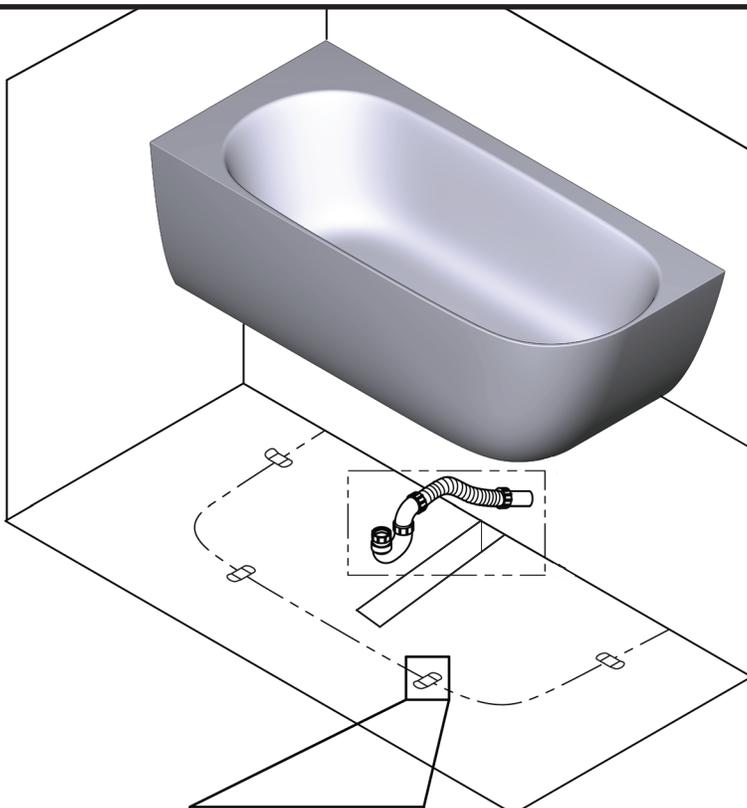
Install bathtub K61 waste drain into floor surface. Position the bathtub spacers (x4) as shown and ensure bathtub drain hole is aligned with waste drain before positioning bathtub.
