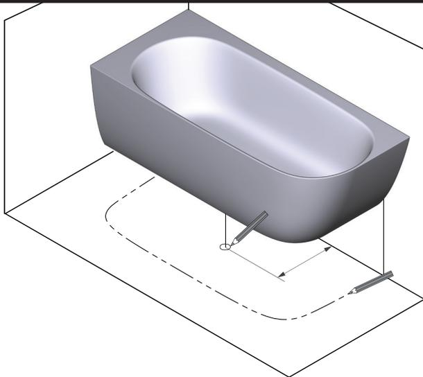
Prepare bathtub floor surface by tracing bathtub bottom edge for installation position.
