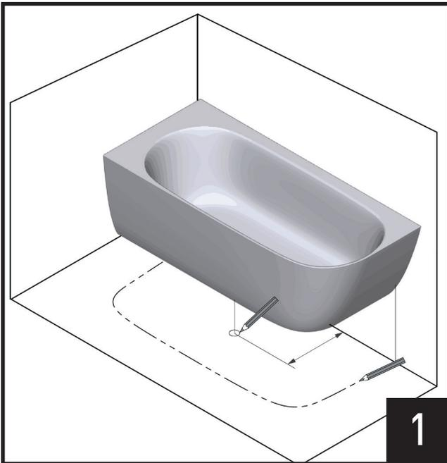
Prepare bathtub floor surface by tracing bathtub bottom edge for installation position.
