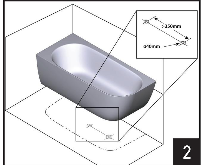
Mark accordingly on floor surface for appropriate waste drain installation connections. Note the inset diagram for waste drain measurements.
