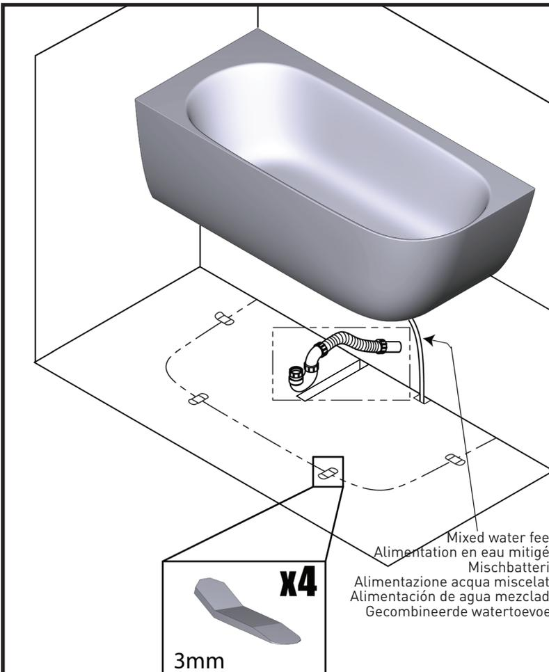
Install bathtub K61 waste drain into floor surface. Position the bathtub spacers (x4) as shown and ensure bathtub drain hole is aligned with waste drain before positioning bathtub.
