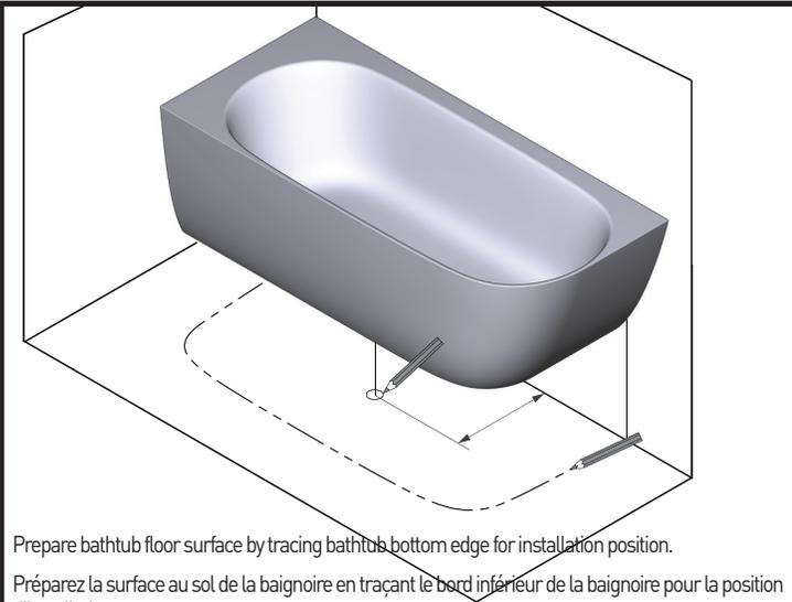
Prepare bathtub floor surface by tracing bathtub's bottom edge for installation position.
