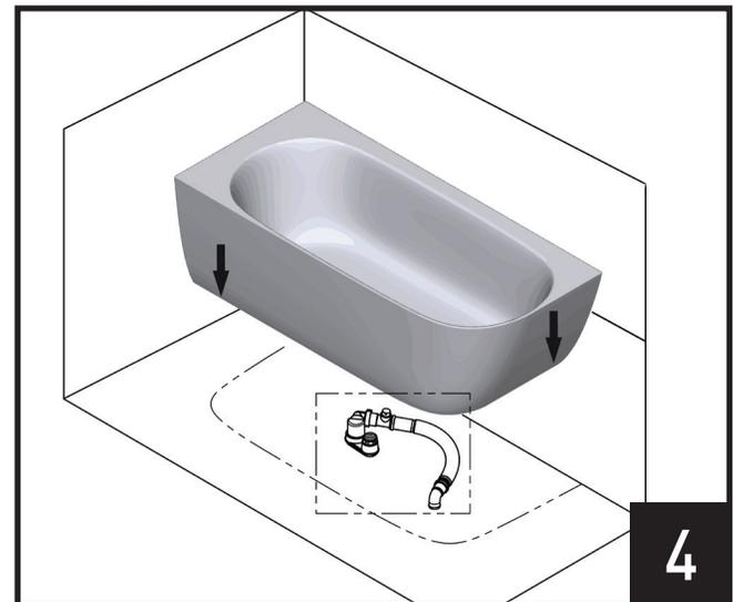
Install bathtub K36 waste drain into floor surface. Install bathtub and align drain with floor waste drain.
