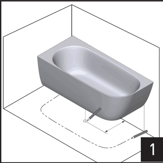
Prepare bathtub floor surface by tracing bathtub bottom edge for installation position.
