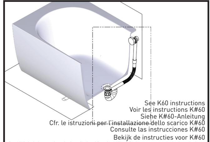
See K60 drain instructions for installation. Victoria + Albert Baths recommends the installation of an access panel for maintenance and repair.
