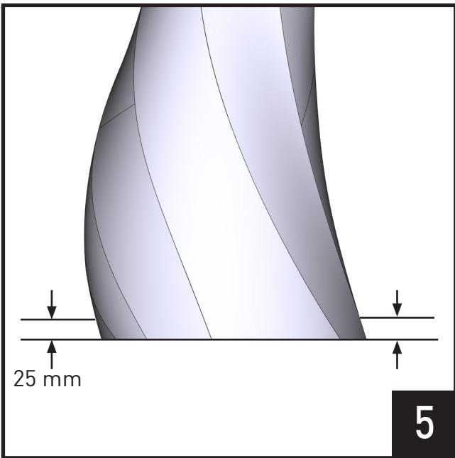
Note the orientation of the basin and the position of the fixing brackets. Supporting the podium, measure and mark out the positions shown in the illustration. Drill a 4mm diameter hole through the wall of the podium basin.
