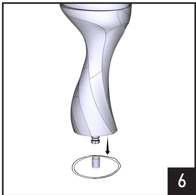
This step will require two people to support the basin. Connect the flexible waste pipe to the waste pipe in the floor. Test waste connections for leaks.
